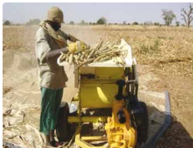
In order to meet quality standards established by the P4P program, farmers must improve on traditional post-harvest processing. Here the "Bamba Thresher", developed in Senegal, is being tested with millet in Mali.
